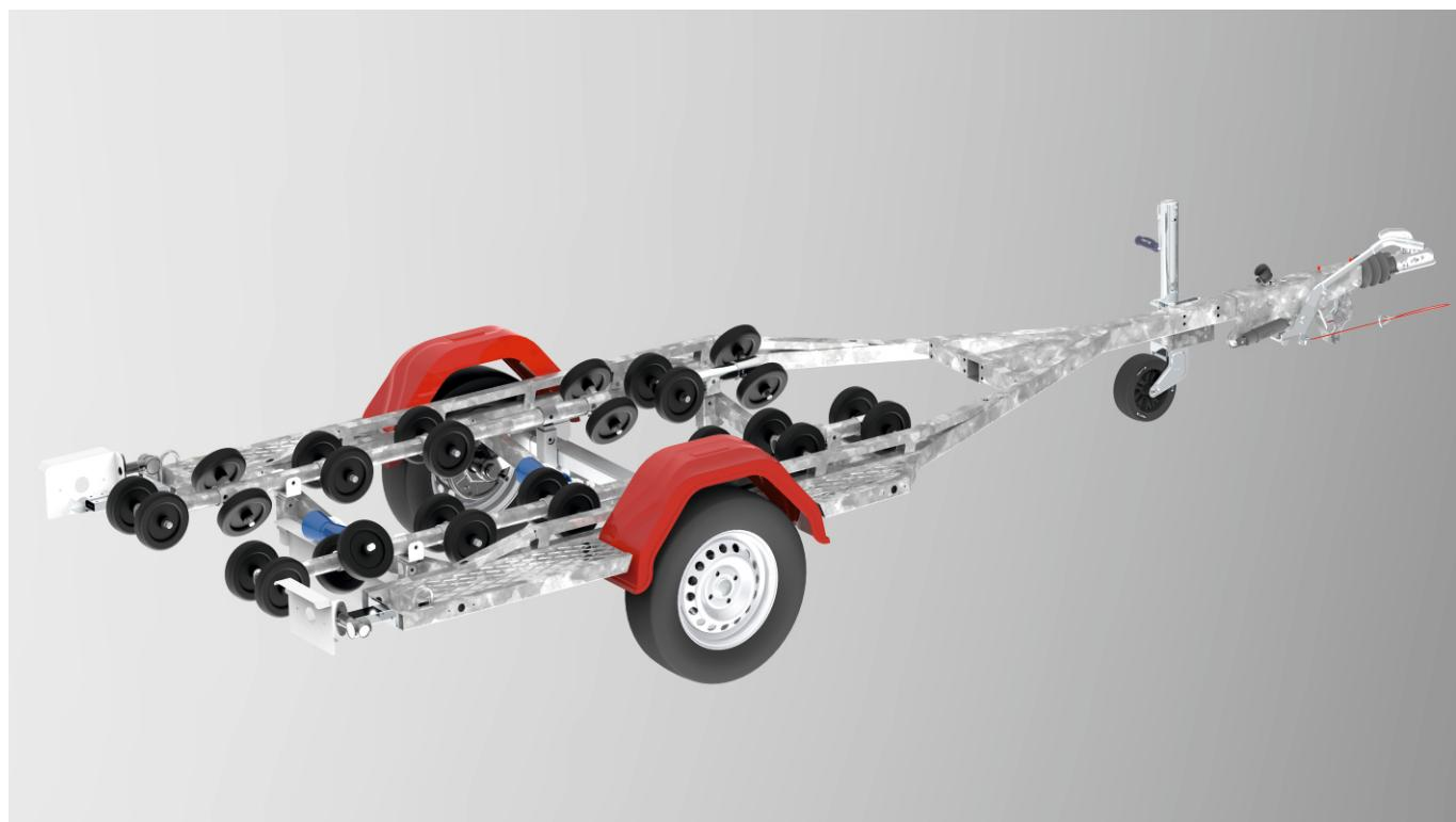
The joining step between the mudguards is an option that will be available early next year
