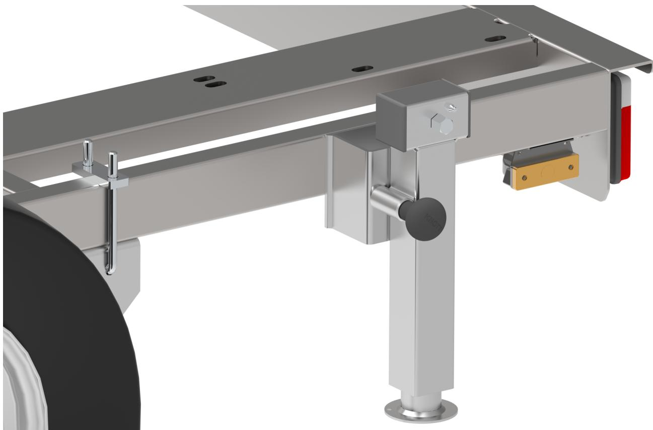
Above, the support is turned to work. This solution reduces the required support stroke, which gives us greater strength with smaller cross-sections
