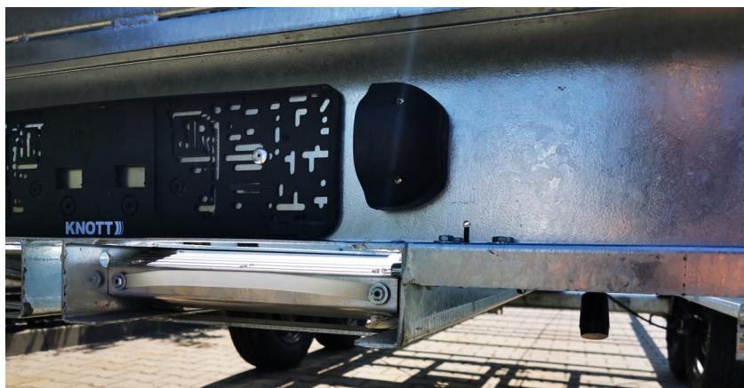
Ramps mounted under the loading surface of the tow truck can also be very easily secured when driving with a trailer.
