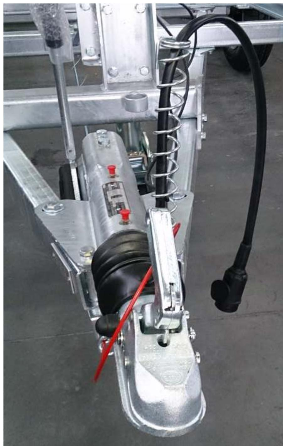
The spring is made of steel and protected against corrosion by galvanic zinc.
