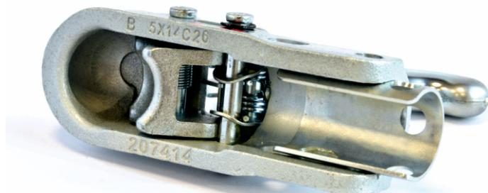
A K30U coupling with a diameter reduction inside. It allows mounting the hitch on sliders with smaller diameters than the nominal one.
