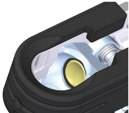
1. Remove worn parts with a hammer and drift
