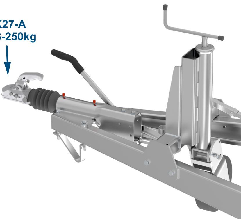
The K27 coupling head is adapted to work with overrun devices with a slider diameter of 50mm and 45mm. Attaching to the breech by means of bolts M12 / M12
