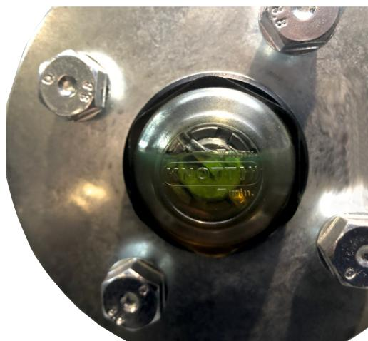
Oil level indicator, thanks to which we can check the amount of oil at any time.
